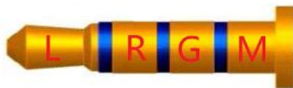
Figure 17 Definition of four-segment headphones
